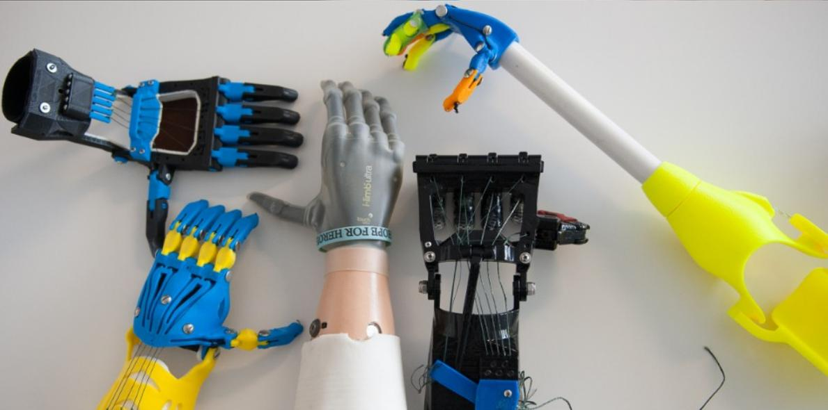
Because prosthetics are such personal items, each one has to be custom-made or fit to the needs of the wearer. AM technology is now regularly being used to produce patient-specific components of prosthetics that match perfectly with the user's anatomy. The ability to produce complex geometries from a range of materials has resulted in AM being adapted at the locations where prosthetics are in contact with a patient.
