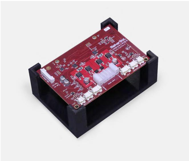
ESD (Electrostatic Dissipative) is a property that reduces static electricity in order to protect electrostatic-sensitive devices, or to contain flammable liquids or gases. Through modifications in chemistry, and the addition of a solid particle such as Carbon Black, 3D printing base polymers, such as PETG, can take on ESD characteristics, making them ideal for creating test fixtures or housings for circuit boards.
